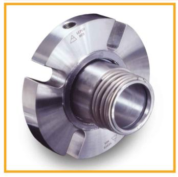
The SEPCO® HOS is a rotary designed, balanced, single spring seal capable of handling higher operating pressures and temperatures than conventional unbalanced single spring designs. Large coil springs are resistant to clogging and allow the HOS to operate successfully in hot oil applications. The seal is available for fitting both standard and oversized seal cavities.
